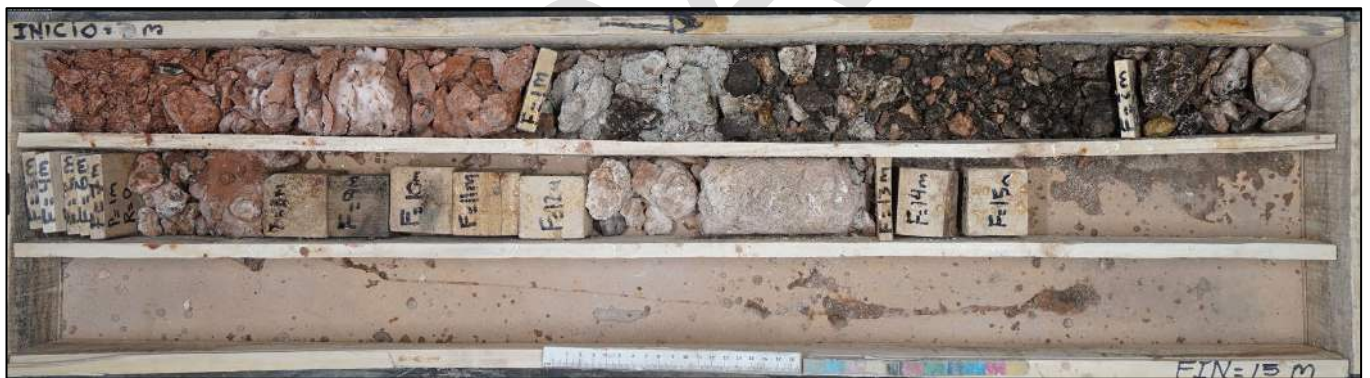
Figura C 2: Sondeo BH-02 0-15 m
