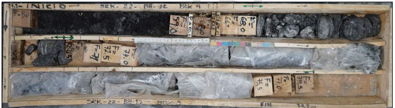
Figura C 18: Sondeo BH12 57.5-79.5 m
