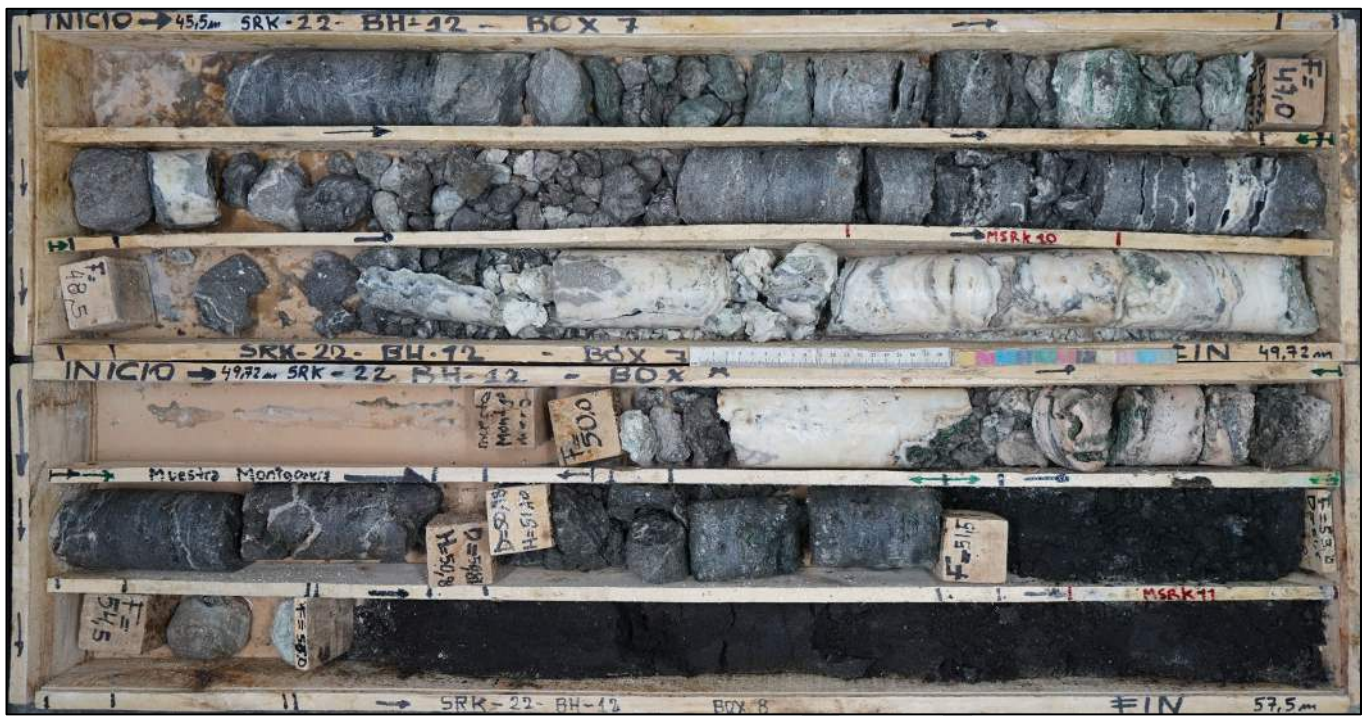
Figura C 17: Sondeo BH12 45.5-57.5 m
