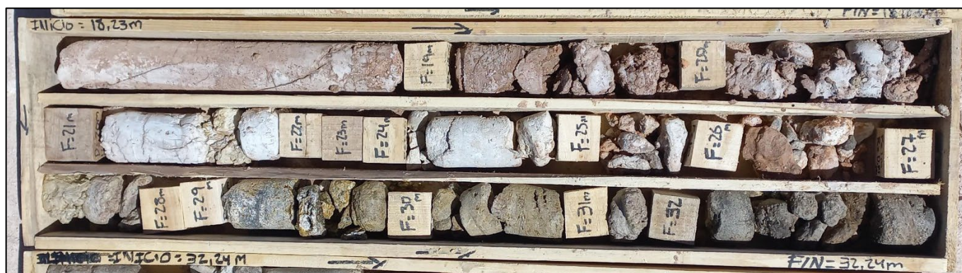
Figura C 27: Sondeo BH16 18.23-32.24 m
